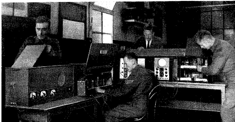
Part of the Basic Training Laboratory at Loughborough College, showing two faulty receivers and one of the faulty transmitters undergoing training repair. A signal generator and a multi-range meter are being used as test instruments with the receivers and an oscilloscope with the transmitter.
